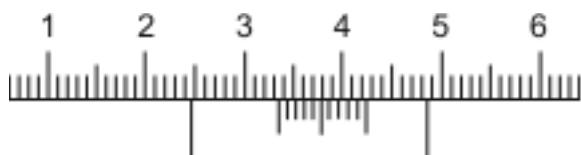
7. a. Read the following micrometer measurement. The micrometer is calibrated in metric units. (1 mark)
